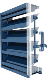
The EXA-645 design features stationary drainable louver blades to protect against water penetration and an integral airfoil blade control damper to allow positive shut-off of air intake and exhaust openings.
